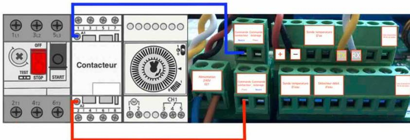
Lastly make the electrical connection of the box EZ1 on a 10A independent circuit breaker on the electrical panel.
